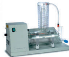
Water Distillation Tank
